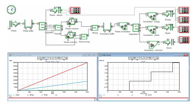
Fig. 3. Simulation model of waste incineration activities in the case study company with a focus on energy, steam, and dioxins.
