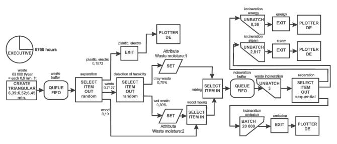
Fig. 2. Block diagram for the simulation system EXTENDSIM showing the incineration process activities within the case study company.
