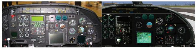
Figure 5 Instrument panel of the AgustaWestland 109 K2 helicopter and as seen in FlightGear
