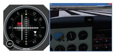
Figure 4 Visualization of the 3D model movements of the indicator on the left, and the actual event during flight as by the FlightGear on the right
