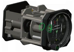
Figure 3 The three-dimensional dynamic model of the KI206 indicator developed in Creo Parametric
