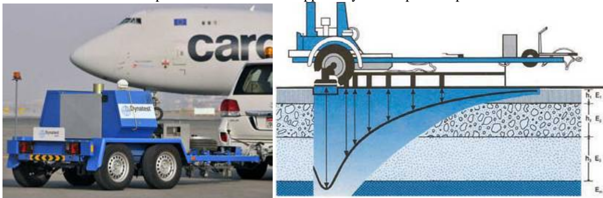
Figure 1 Typical HWD and this application on pavements
