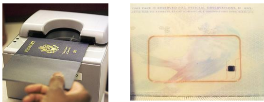
Figure 6 Biometric Passport Reader and RFID Chip in a Passport [18]
