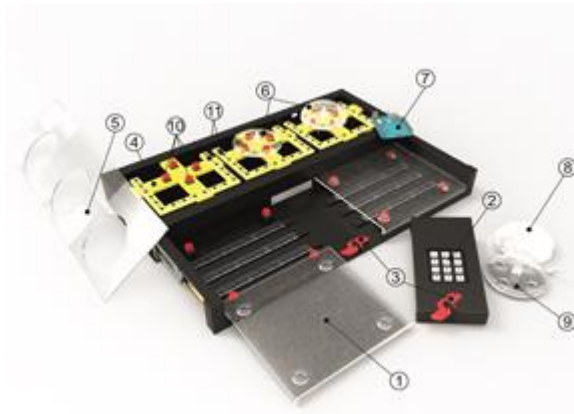
Fig. 1 Device visualization as USB box decomposition with sliding touch plates. 1 - touch plates; 2 - numeric keyboard; 3 - electromyographic measurement unit; 4 - frame; 5 - cover; 6 - buttons; 7 - control unit; 8 - button cover; 9 - connection element; 10 - micro switches; 11 - LED strips.
