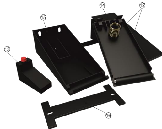
Fig. 2 Pedals decomposition. 12 - pedals; 13 - sliding block; 14 - pushing spring; 15 - device cover; 16 - connecting slat.
