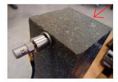
Figure 9. Location of the vibration acceleration sensor indicating the direction of stroke.
