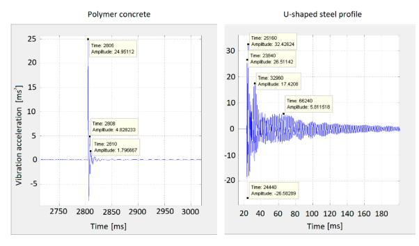
Figure 13. The comparison of damping in polymer concrete and U-shaped steel profile.
