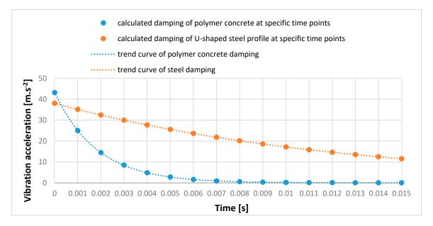
Figure 14. The comparison of calculated damping of polymer concrete and U-shaped steel profile.
