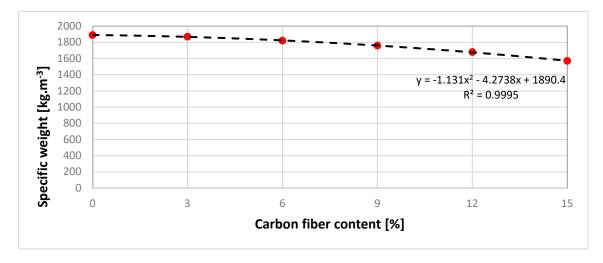
Figure 12. The graphical comparison of the effect of the carbon fiber content on specific weight.
