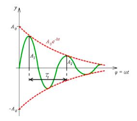
**Figure 10.** The schematic representation of attenuation  $\lambda$  in muted oscillation motion.
