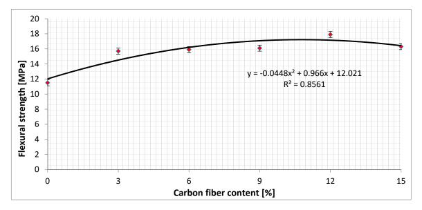
Figure 11. The graphical comparison of the effect of carbon fiber content on flexural strength.
