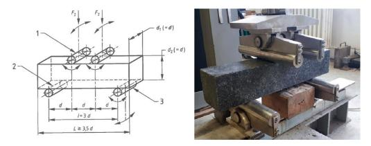
Figure 7. Test sample mounting scheme.
