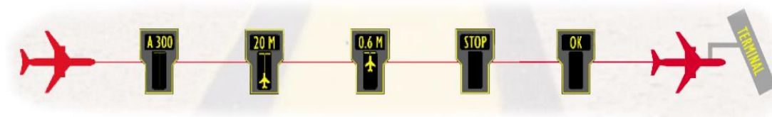
Figure 3 Honeywell parking system
